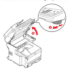
**3.** Press the cover release (a) and open the top cover (b) fully.
